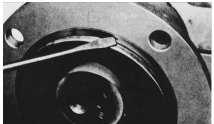
Figure 4.3. Typical Retaining Ring Removal
